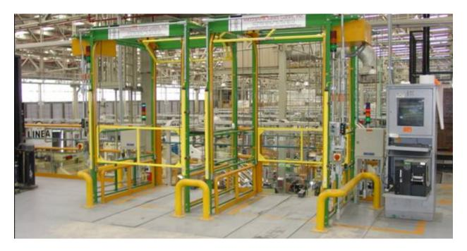
Two Roly safety gates feature power operation with stations for push-button operation. A fork-lift truck is able to open the safety gates from below with a radio frequency remote.
