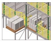
The Pallet Flow Pick Module Swing Gate provides protection in high bay rack picking areas
