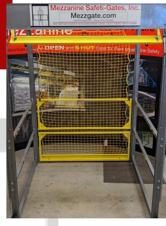
When the pallet drop area is being loaded, the ledge gate is open and the netting compacts into the system, clearing the way for pallets to be moved into place. After loading is finished and the pallet area is ready for picking, the ledge gate closes and the netting extends from the deck to the top frame of the gate, providing full length coverage to prevent products from falling, decreasing the risk of damage while being picked or moved from the area.
